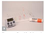
Place a new Reveal for Ochratoxin strip into the sample cup. Set a timer for 9 minutes.
